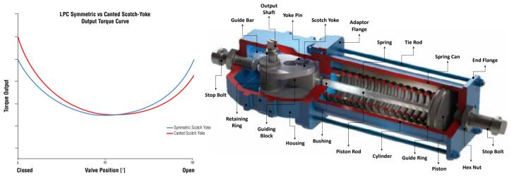
Detailed Output Torque Characteristics are available for both Spring Return and Double Acting executions.
